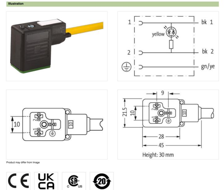
Cable length 10 m Side 1 0,4 Nm Tightening torque The information in this Product-PDF has been compiled with the utmost care. Liability for the correctness completeness and topicality of the information is restricted to gross negligence. Version: 2024-05-04
