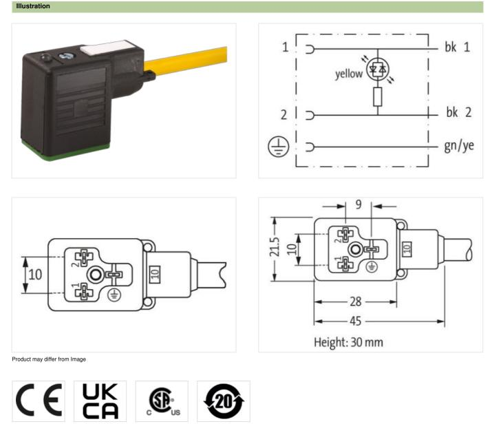
Cable length 10 m Side 1 0,4 Nm Tightening torque The information in this Product-PDF has been compiled with the utmost care. Liability for the correctness completeness and topicality of the information is restricted to gross negligence. Version: 2024-05-20
