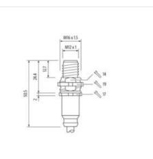
PROFI 「南山ぐ Cable length 1 m Side 1 0,6 Nm Tightening torque
